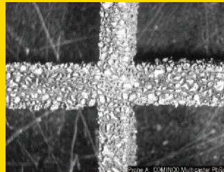
Corrosion layer of new alloy
